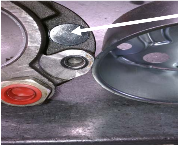
Pump Housing before reservoir installed. Note Magnet on housing to catch metal particles.
